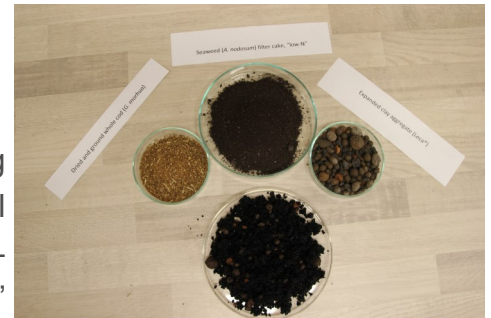
Example of a compost mixture: Algae fiber, fishmeal, and Leca.
